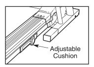
justment knob counterclockwise. To decrease the firmness, turn the knob clockwise. **Note: The faster you run on the treadmill, or the more you weigh, the firmer the cushioning system should be.**
